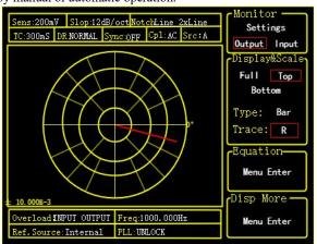
synchronous filter can be used to eliminate the influence of the harmonics of the reference signal, ensuring that OE1022 can detect a low-frequency signal quickly and effectively.
